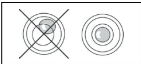
Note: Regularly check whether the instrument is in a level.
